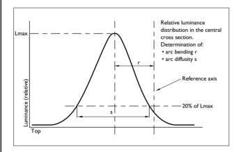
Vertical Luminance cross-section at centre of the arc: measured at 27.1mm from reference plane
