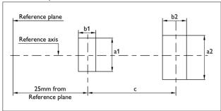
This test is used to determine whether the electrodes are correctly positioned relative to the reference axis and the reference plane.
